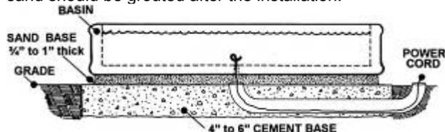
• It is recommended to place a sweep of 2" conduit or PVC underneath the basin from the center out to the edge or to the power source prior to installing the fountain. This will prevent major dismantling should the pump need to be replaced by stringing the pumps power cord through the conduit. Please consult an electrician regarding local code requirements. Most pumps supplied by AI's Garden Art come with a minimum 15-foot power cord and requires
